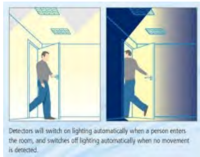
Figure 4: How Occupancy Sensors Work
